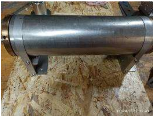
Submersible type core holder.
