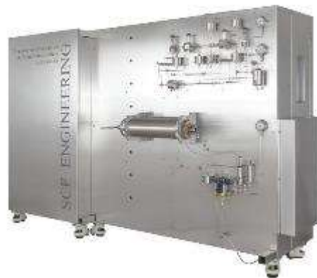
Fig. 4. SKIF-FSK lab equipment for filtration experiments on core samples.
